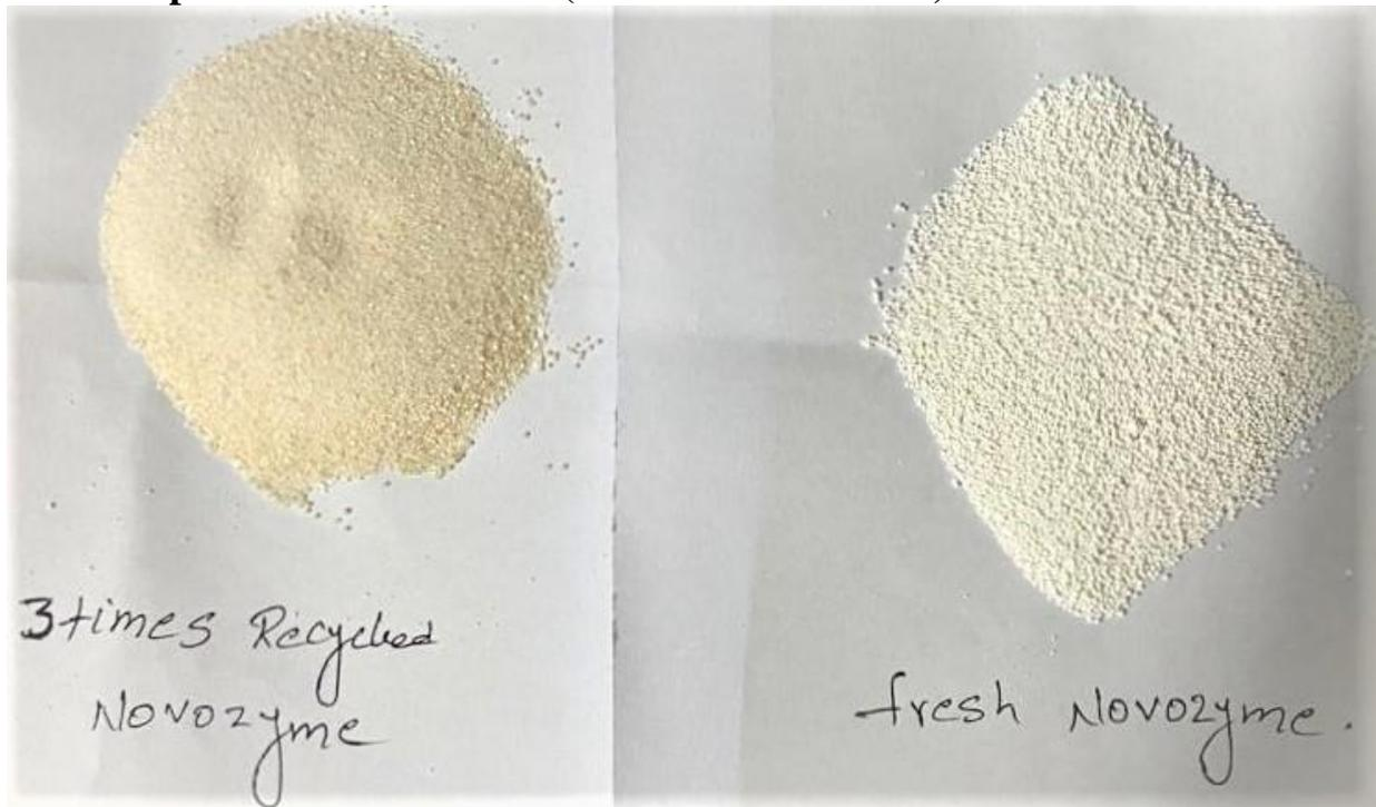
This observation shows, Novozym-435 could be recycled three times but slowly it was transforming to powder like material and hence conversion to EIDD and diacylated EIDD was affected (94% vs 86%).
